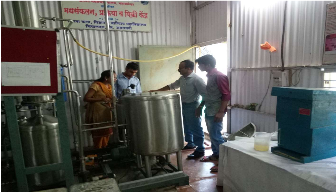
Demonstration of feeding of raw honey to feeding tank of honey processing plant.
